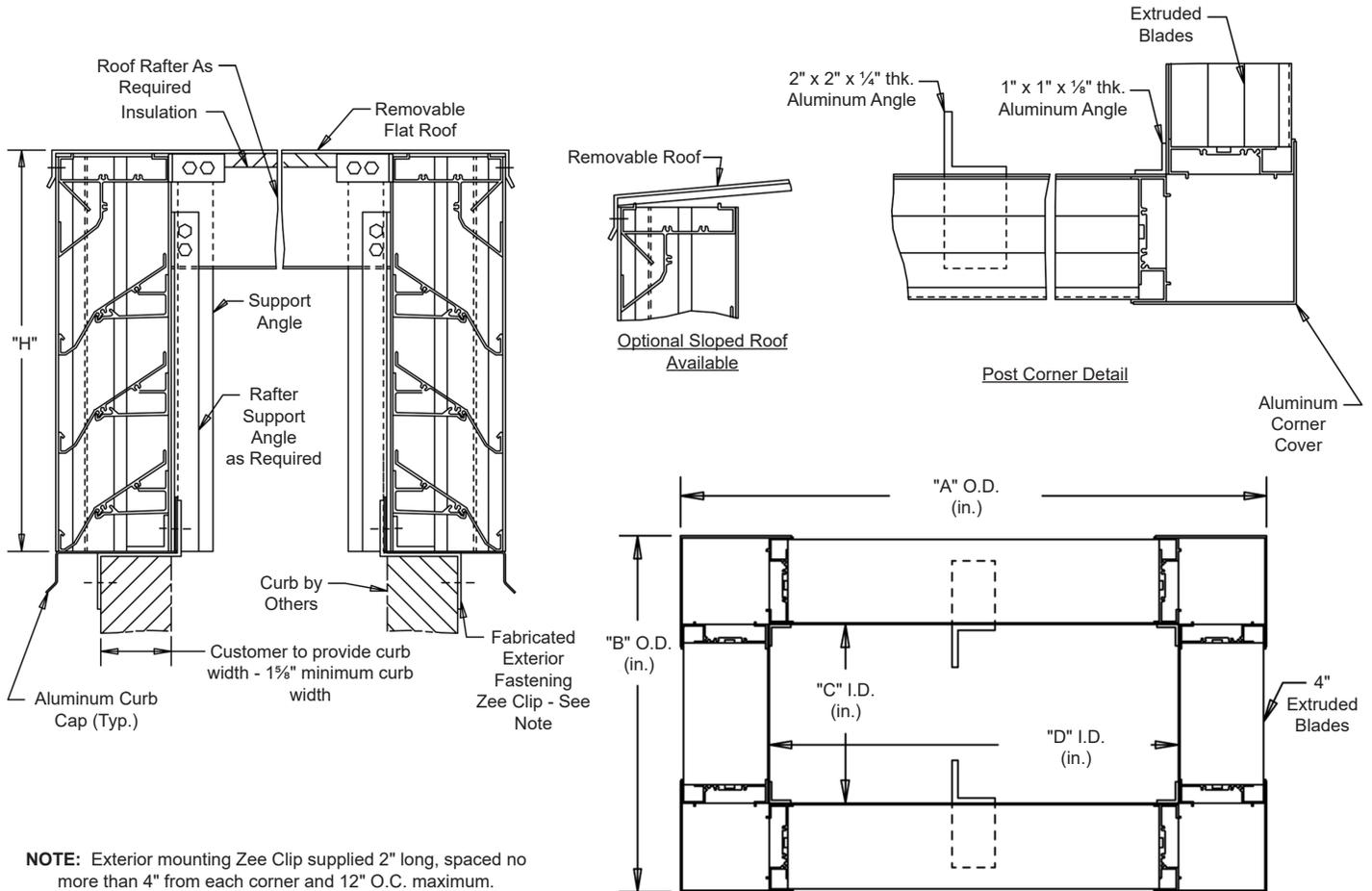
**NOTE:** Exterior mounting Zee Clip supplied 2" long, spaced no more than 4" from each corner and 12" O.C. maximum.
